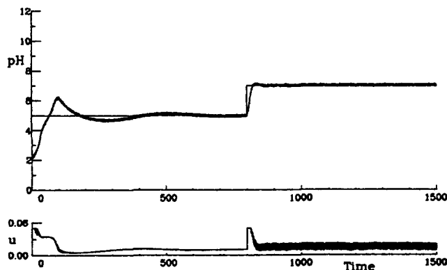
Figure 6. Control performance for process iii with measurement noise of \pm 0.1\text{pH} .
